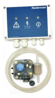
The Airflow Alarm monitors pressure conditions in a duct. A pressure switch connected to the control box provides the signal input.
