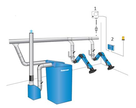
Airflow alarm and pressure switch mounted
