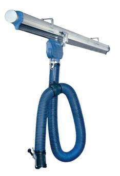
Efficient system for trucks, cars and vans in motion. With damper and shock absorber on trolley and safety coupling on exhaust hose for maximum operational safety. Available with automatic disconnection of the nozzle. The 920/1500 trolley is specially designed for moving vehicles. The maximum design airflow is 1500 m<sup>3</sup>/h (880 cfm) per trolley.
