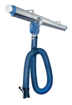
Efficient system for trucks, cars and vans in motion. Includes balancer, damper and shock absorber on trolley and safety coupling on exhaust hose for maximum operational safety. Available with automatic disconnection of the nozzle. The 920/1500 trolley is specially designed for moving vehicles. The maximum design airflow is 1500 m³/h per trolley.
