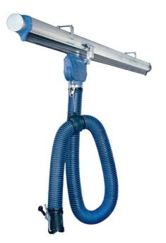
Efficient system for trucks, cars and vans in motion. Includes balancer, damper and shock absorber on trolley and safety coupling on exhaust hose for maximum operational safety. Available with automatic disconnection of the nozzle. The 920/1500 trolley is specially designed for moving vehicles. The maximum design airflow is 1500 m<sup>3</sup>/h per trolley.
