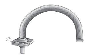
Extractor arms for use in electonic industries, laboratories, schools etc. Flexible plastic hose with a very good resistancy against solvents etc. Stays in new position when adjusted. ESD safe. Swivel with 360 degree rotation. This means that the connected ductwork remains firm and does not rotate with the arm. Mounting directly in bench surface or with accessory brackets. Can be mounted both standing and hanging.
