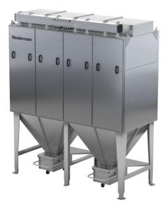
MCP SmartFilter Ex is a multi-purpose filtration system. It is customizable to perfectly fit customer specific demands with airflow up to 28 000 m3/h. Suitable for smoke, fumes, dust and combustible dust and can be used in several different applications such as welding, metal cutting and general dust.
