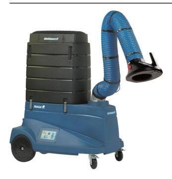
The FilterCart Advanced+ is a light-weight, portable and easy to manoeuvre dust and fume extractor with a warning signal when the filter is full. It includes an easy-to-position Original extraction arm with an extended working range, thanks to the 10 ft. (3 m) long arm. The arm is already fitted to the unit enabling a fast and easy setup. The disposable nanofiber filter offers both significantly longer filter life and higher efficiency than previous versions of the FilterCart.
