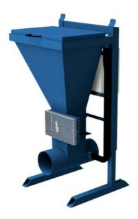
The lime feeder type NFKG-70 contains approximately 70 kg of lime and is equipped with a level indicator which indicates shortage of lime. The lime feeder feeds approximately 15 g of lime per movement, depending on the humidity of the lime.
