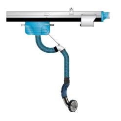
The MAX Rail exhaust solution is designed with the market proven MagnaRail track and trolley system and our new MAX Nozzle. The MAX nozzle connects directly to a robust adapter secured to the vehicle tailpipe and disconnects as the vehicle exits the bay. Features a patent pending design that induces ambient air to cool both the airstream and connection magnets reducing wear and tear and maintenance needs for the system.
