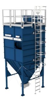
LCP SmartFilter is a heavy-duty multi-purpose filtration system. It is customizable to perfectly fit customer specific demands, with airflow up to 50 000 m3/h for standard version. Suitable for smoke, fumes and dust and can be used in several different applications such as welding, metal cutting and general dust and process filtration.
