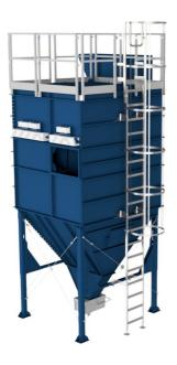
LCP SmartFilter is a heavy-duty multi-purpose filtration system. It is customizable to perfectly fit customer specific demands, with airflow up to 50 000 m3/h for standard version. Suitable for smoke, fumes, dust and combustible dust and can be used in several different applications such as welding, metal cutting and general dust and process filtration.
