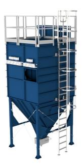
LBP SmartFilter is a round bag filter designed for continuous operation in many industries, for virtually every kind of process and nuisance dust. It is customizable to perfectly fit customer specific demands, with 3 different bag lengths, filter area up to 266m2 and airflow up to approx. 30.000 m3/h (depending on duct characteristics).
