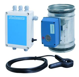
The motor damper consists an operation box that can be controlled by any closing switch. The operation box consists of a 30 VA transformer for the lighting kit in the extraction arm, a delay timer for fan stop variable from 0-5 minutes, and two separate connections for sensor clamps.
