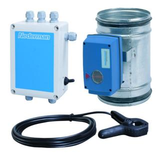
The motor damper consists an operation box that can be controlled by any closing switch. The operation box consists of a 30 VA transformer for the lighting kit in the extraction arm, a delay timer for fan stop variable from 0-5 minutes, and two separate connections for sensor clamps.
