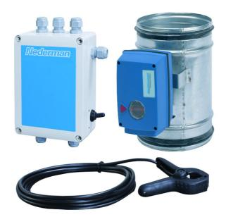
The motor damper consists of a fan switch and an operation box that can be controlled by any closing switch. The operation box consists of a 30 VA transformer for the lighting kit in the extraction arm, a delay timer for fan stop variable from 0-5 minutes, and two separate connections for sensor clamps.
