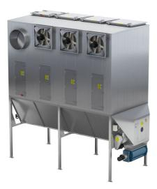
The LBR-C is an advanced, IIoT ready, reverse air baghouse suited for continuous duty applications with high air volumes and heavy dust loading. The modular filter housing can be scaled for the required airflow and additional modules can be installed in the field if additional capacity is required. The LBR filter is self supporting with telescopic legs for height adjustment and is suitable for outdoor installations.
