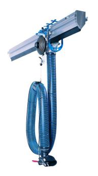
ALU 150/250 is an advanced exhaust rail system for high frequency use. The ALU 150/250 offers a large number of features, such as manual return of extraction units on a separate track, automatic disconnection of nozzles and balancer. NB! When using a straight rail solution one hydraulic limit stop (see accessories) must be attached in the end of the rail system.
