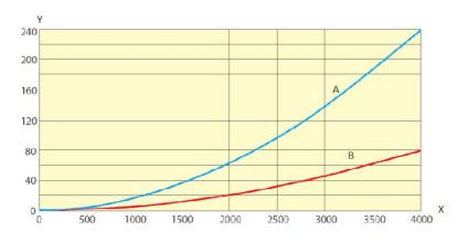
Y= Pressure drop (Pa), X= air flow (m3/h) A = ALU Ø150 mm B = ALU Ø250 mm
