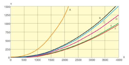
Y= Pressure drop (Pa), X= air flow (m3/h) A = Trolley fume extractor arm
