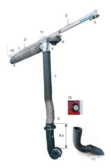
MagnaTrack Green is designed for medium exit-speeds of one vehicle per back-in bay. Can accommodate low level or high level tailpipe vehicles. Mounted on a track system available in lengths of 10 feet or 13 feet for low level tailpipes or 23, 30 or 40 feet for high level tailpipes.
