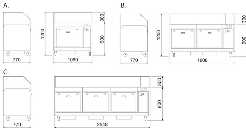
A: FilterBench 23 B: FilterBench 46 C: FilterBench 69
