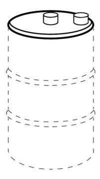
Pre-separator consisting of a steel lid with an inlet and an outlet for connection to the pipe work for pre-separation of coarse material, metal chips and cutting fluids.
