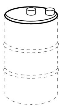
Pre-separator consisting of a steel lid with an inlet and an outlet for connection to the pipe work for pre-separation of coarse material, metal chips and cutting fluids.
