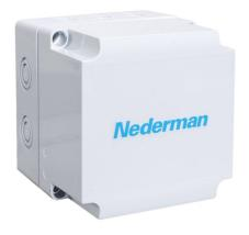
To start/stop a central fan in combination with a number of motor dampers. (Larger capacity fans may be remote controlled via a Nederman fan starter or fan inverter.) The fan switch has motor protection included. Protection class IP66. Coil 24V AC, from operationbox or transformer.
