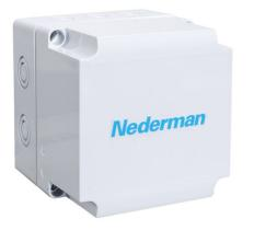
To start/stop a central fan in combination with a number of motor dampers. (Larger capacity fans may be remote controlled via a Nederman fan starter or fan inverter.) The fan switch has fan motor protection included. Protection class IP66. Coil 24V AC, from operation box or transformer.
