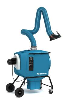
The FilterBox 10A is equipped with a N24 fan for a maximum air flow capacity of 1 000 m3/h (600 CFM). An integrated silencer reduces noise from the fan and outlet air.
