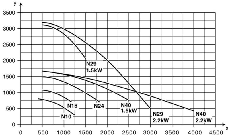
X: airflow, m³/h Y: static pressure Pa
