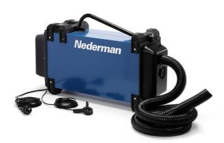
The Fume Eliminator is designed to be carried to the working area. Connected to a welding torch or to an extraction nozzle, the FE unit extracts the fume directly at source. FE 840 has a manual start/stop function while the FE 841 has an automatic start/stop function, which starts the unit as soon as the welding begins.
