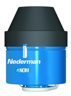
The NOM 4 is an oil mist filter in compact design and therefore suitable for enclosed cabinet single CNC machines. The unit is easy to install and enables maximum flexibility in the workshop, as it is normally installed on top of the machine. The NOM 4 is suitable for emulsion mist.
