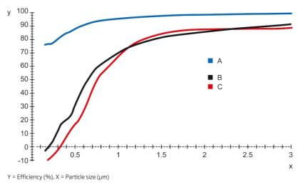
A = NOM filter, B = Centrifugal filter A, C = Centrifugal filter B
