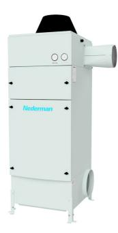
Designed for lathing and milling applications, for machines stamping and pressing steel plates, industrial washing machines, abrasive water jets etc. In all metal fabrication with oil mist troubles, these filters will fit into a ducting system, connected to each machine. All units are equipped with pressure gauge for control of filters as well as an indication for need of cleaning (self draining). Suitable for emulsion mist.
