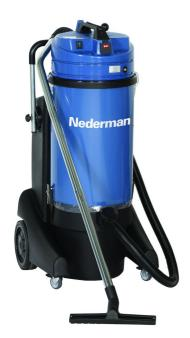
The 300E is a compact industrial vacuum cleaner with long filter lifetime, 4000 - 6000 hours with bag filter. This dry vacuum is robust but easy to transport and has micro-filter as option. Convenient accessory box for brushes, nozzles etc. on the rear of the unit. Optimal suction power – twin single phase motors.
