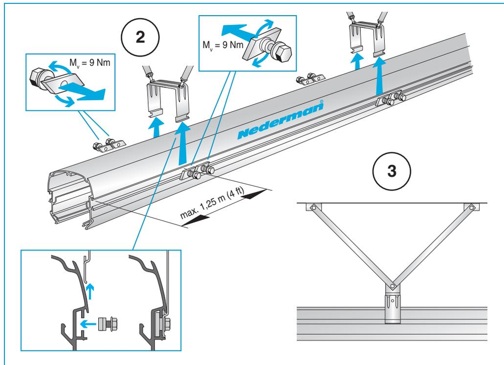
Joining rail sections
