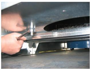
15) Unscrew the nuts securing the fan to the base. Access via the fork lift entry.
