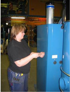
4) Remove the rear panel. Note! Unscrew the lower screw securing the panel to the base plate. Screw is accessed via the opening for the forklift.
