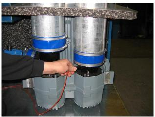
8) Unscrew the gland nut and remove the PT100 sensor rod.
