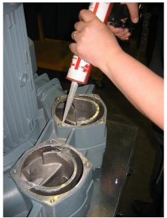
20) Apply the sealant shipped with the new pump. The sealant is a high temperature, silicone free sealant.
