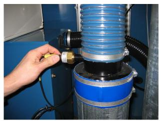
5) Disconnect the pressure transducer
