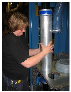
23) Refit the silencers and tighten the hose clamps.
