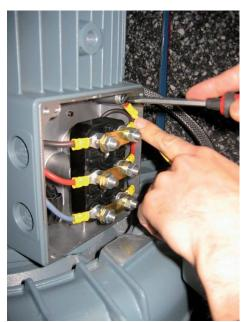
29) Re-connect the power supply to the motor. NOTE! Ensure that the cable gland have contact with the cable shielding.
