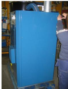
30) Refit the rear panel. NOTE! Refit the lower corner screw.
