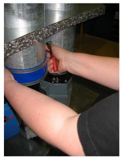
11) Remove the upper hose clamp between the adapter and silencer pipes.
