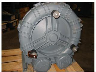
17) Fit the old vibration dampers to the new fan. Do not forget the copper earth plate.
