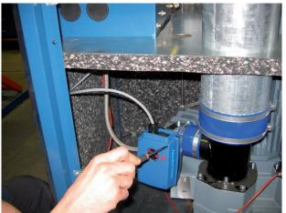
7) Remove the vacuum valve cover, and disconnect the wires. Note! Mark the position of the wires for correct re-assembly.
