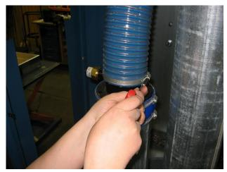
10). Loosen the hose clamp and disconnect the flexible hose from the inlet silencer.
