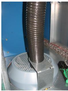
28) Fit the flexible hose to the bracket. Ensure that the hose is pushed flush against the motor grid/cover.
