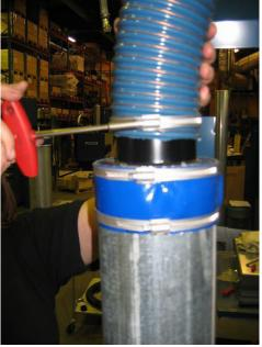
24) Refit the flexible hose to the top of the intake silencer. Note! Ensure proper grounding by tightening the copper wire against the unpainted area of the adapter.
