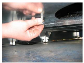
19) Secure the new fan to the base.
