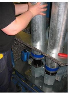
12) Remove the two silencers (up and out).
