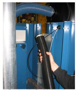
6) Remove the flexible hose between the motor and inverter housing
