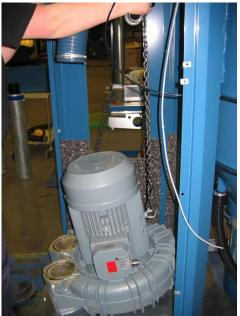
16) Carefully lift the fan out. Pay attention not to damage the vibration absorbers as they will be reused (NOTE! Fan weight: approx 130 Kg).
