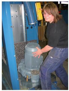
18) Fit the new fan into position.
