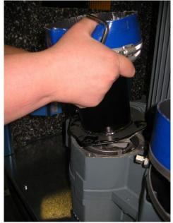
14) Unscrew and remove the two adapters for the silencers. Remove the remains of the sealant.
