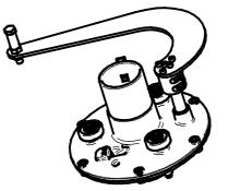
1. Replace the old damper housing with the new.
