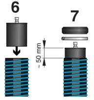
Put the male part of the safety coupling in the lower hose, approximately 50 mm out from the hose end.
