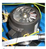
6 Unscrew the plastic cover of the motor (2 screws).
