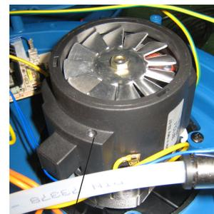
**6** Unscrew the plastic cover of the motor (2 screws).
