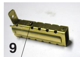
Bend this tap upwards on the new carbon brush to make the carbon pop out from the brass housing.
