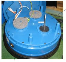
5a Remove the rubber rings (one at each side).
