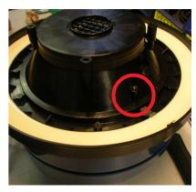
The micro-filter must be positioned with the gash coming over the part directed outwards on the suction top.
