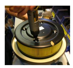
Secure the micro-filter with screws and remove the piece of tape.
