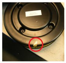
Put a piece of tape on the top of the micro-filter to know where the gash is when mounting.
