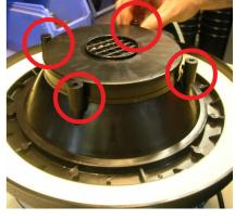
Position the new distance sleeves (enclosed with the new micro-filter) on the suction top.
