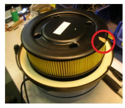
The micro-filter must be positioned with the gash coming over the part directed outwards on the suction top.
