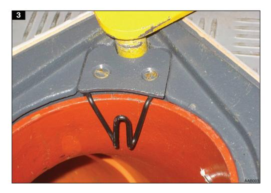
The safety belt is hooked into the safety hook. See figure No. 4.
