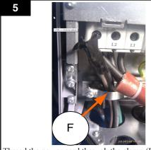
Thread the power cord through the clamp (F).
