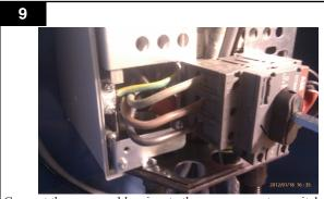
Connect the power cable wires to the emergency stop switch. Make sure to only clamp the wire and not its insulation, which creates a poor contact and damages both the power cable and the emergency stop switch.
