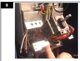
Replace and secure the emergency stop switch (B).
