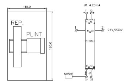
Connect input voltage 24 V - 230 V to terminals 1 and 2.
