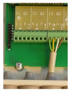
Each output has an automatic software check to protect against the valve wires becoming short-circuited. At currents above 4 A<sub>peak</sub> an active output will toggle on and off to avoid overheating. This operation protects the outputs and the power supply until the short has been removed. The fault is reported back to the PC for correction. The protection, however, does not cover all types of wiring errors, so please check the installation carefully before starting the unit.
