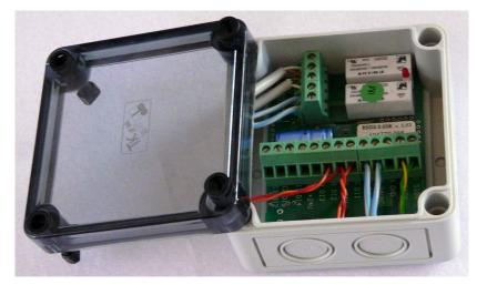
The wires to the taps connect to 6 and 7 (tap 1) and 8/10 and 7, (tap 2).
