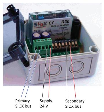
The secondary side is connected to terminals 11 and 12. 11 is internally connected to (the Ground) terminal 4, making the secondary bus half susceptible to involuntary connections between the supply and bus at other I/O-units.
