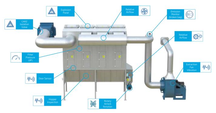
Sensors monitor component operation that are critical to safety and performance and then connect to the Insight Control panel where data is securely uploaded to the Insight IIoT System (optional).
