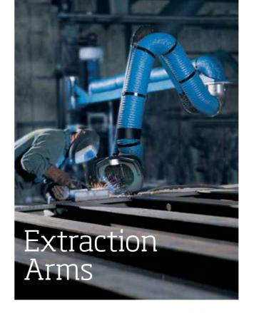
Extraction arms are the welder's primary interface with fume extraction systems and therefore the design, quality and performance are vital for reliable and effective capture. Nederman's best-in-class extraction arms are designed to optimize fume capture, easy to operate and reliably hold their position so frequent adjustment is not required. The arms are durably constructed in order to handle the challenges associated of welding environments.
