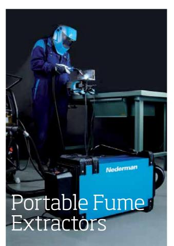
Portable fume extractors are on-torch capture devices designed to go wherever welding needs to be done. These are great solutions for light production welding especially in tight spaces (confined space) where it would be difficult to use extraction arms. They are also great to have in maintenance departments or on-site repair work and can ben conveniently kept in service vehicles and carried onto construction sites.
