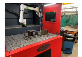
Fume extraction at the torch for cobot workstation with FE GoMax
